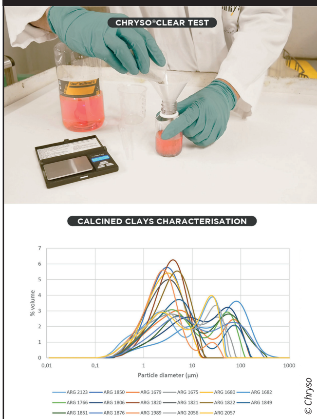
Figure 1: Using Chryso's proprietary Clear Test, the R&D team worked on the characterisation of over 30 calcined clays, originating from around the world
